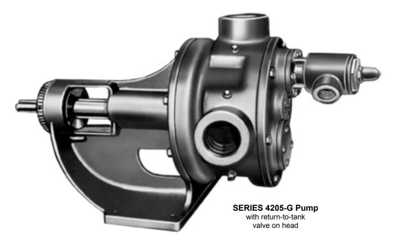
The series 4205-G above illustrates the basic pump construction for LP-Gas Truck Pumps and Units ("R" and "V" Drives.) The pumps are equipped with return-to-tank bypass valves on heads, or on request, internal relief valves can be substituted for the return-to-tank valves (see Section 630, Page 630.2) Simple, dependable mechanical seals, leak-proof O-Ring gaskets, internal pressure lubrication system, integral thrust bearings
