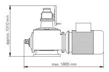
Weight according to equipment (without motor) approx. 750 - 1200 kg
