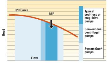
System One<sup>®</sup> pumps resist vibration for a larger operational window off the BEP and greater reliability.
