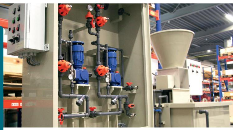
When processing chemicals, high demands are placed on your process with regard to safety for people and the environment. Therefore, AxFlow Systems total solutions for dosing chemicals are carried out entirely in-house in custom-made dosing cabinets to ensure the safety of you and your environment.
