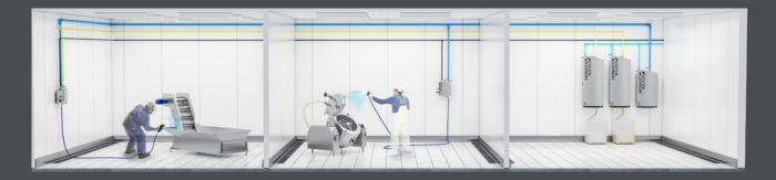
A central solution is characterized by prediluted chemicals being pumped to each workstation from a chemical pump station placed in a separate, central location.
