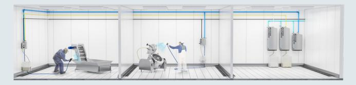
A hybrid solution has the same setup as a central system but with the additional possibility of adding an extra product at all or some of the workstations. The solution is often applied when there is a need for an extra cleaning task to be performed independently of the regular cleaning program.
