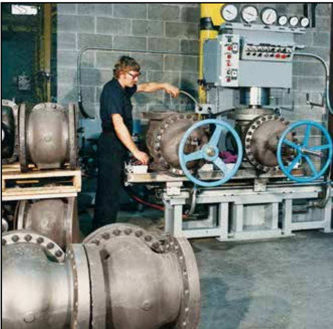
Semi-automatic stations for testing NPS 2-12 (DN 50-300) valves to API 598.
