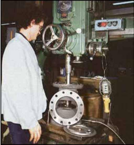
3 Relapping of seating faces after seal welding.
