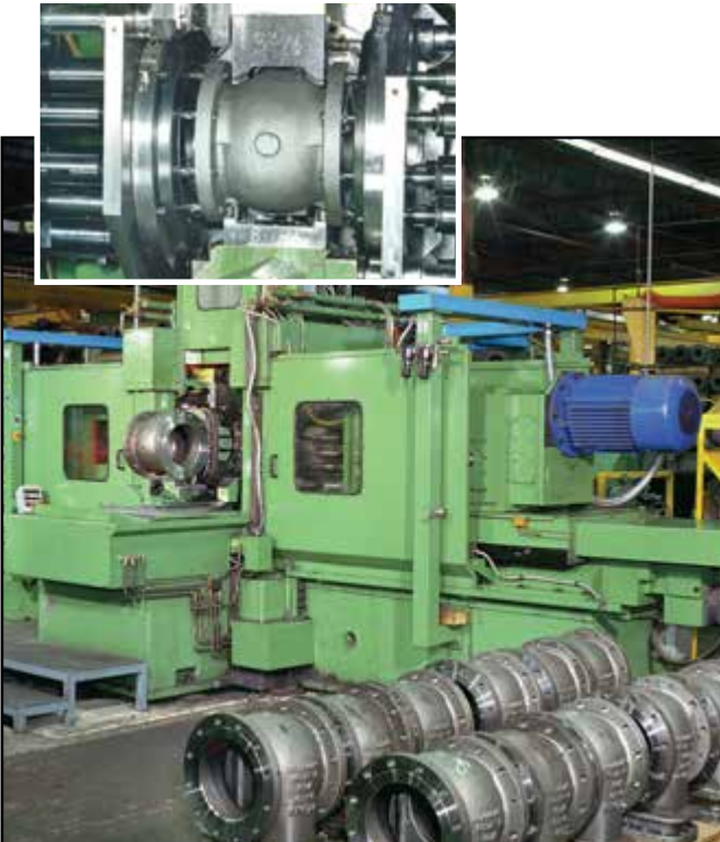
Automatic multiple drilling machine.
