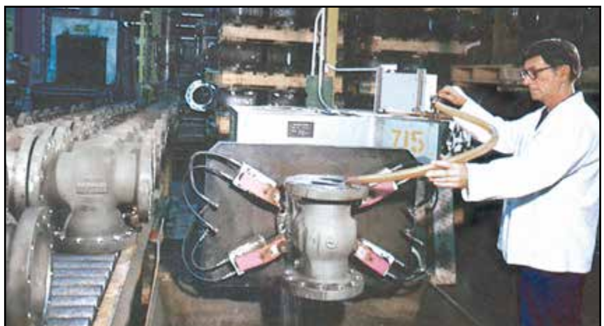
2 Air-under-water test of the seat's welds.
