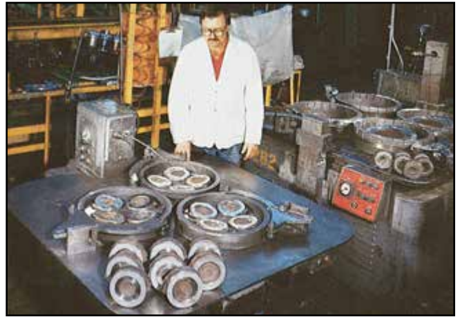
6 Lapping of wedge seating surfaces.
