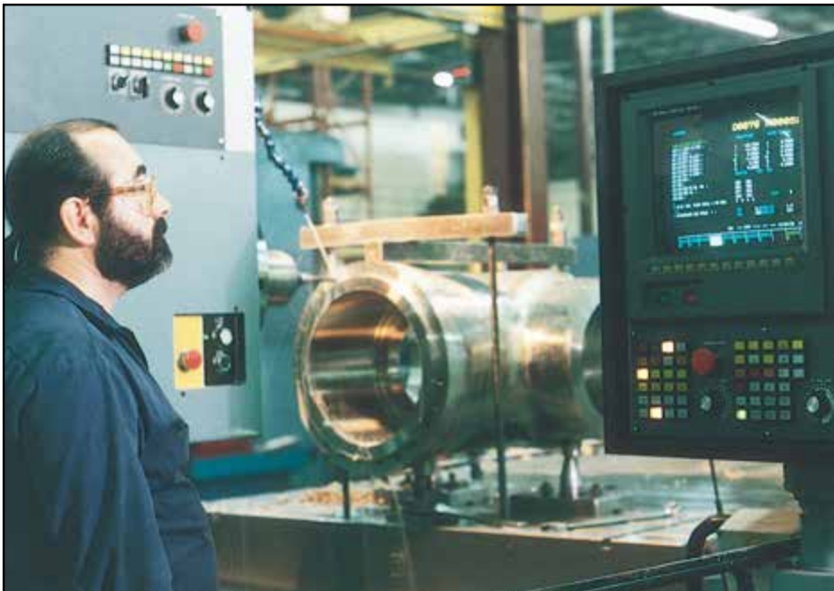
An operator on a CNC horizontal boring mill monitors his own quality.
