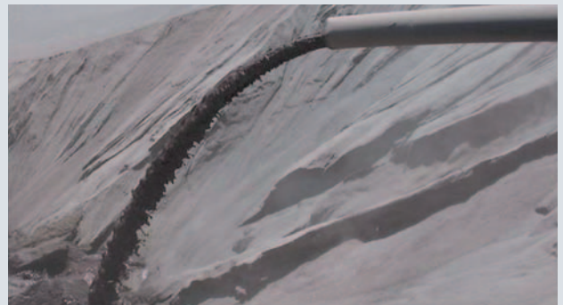
Copper tailings, 60 % solids concentration
