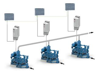
To synchronize multiple pumps, each pump must be equipped with a VFD and PLC Control.
