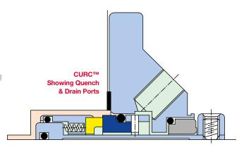
\*A version of the CURC™ can be supplied, with a fully machined gland, which conforms to the dimensional requirements of API 682. These can be used on applications where qualification tested, fully API 682 compliant seals are not required.
