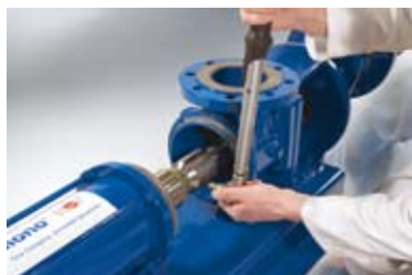
Skruva loss kopplingshylsan
