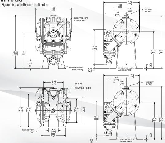
HDB2 & HDB50, Top Ported Dimensions are ± .13" (3mm). Figures in parenthesis = millimeters
