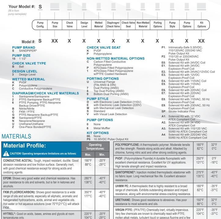
which readily liberate free fluorine at elevated temperatures. Maximum and Minimum Temperatures are the limits for which these materials can be operated. Temperatures coupled with pressure affect the longevity of diaphragm pump components. Maximum life should not be expected at the extreme limits of the temperature ranges.
