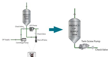
With its high suction capability, the Universal TS Series pump is both process and CIP capable, allowing you to reduce the number of pumps, valves, and control systems in your process and save capital equipment costs.
