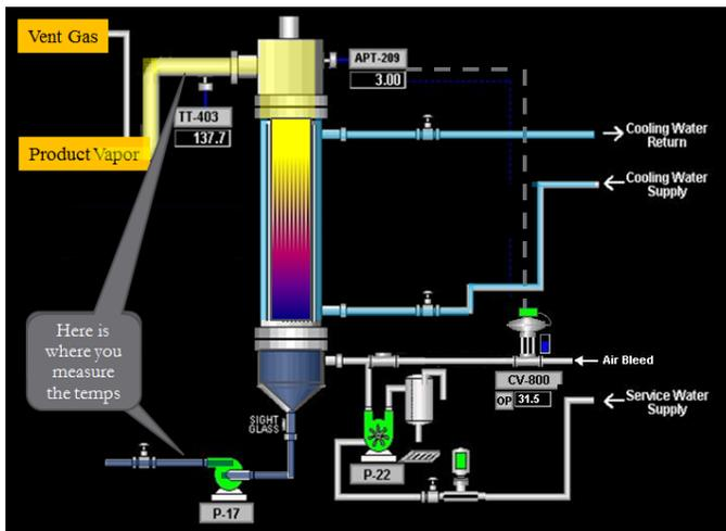
Note that an IR scanner requires a dull surface to measure correctly; a reflective surface such as stainless steel will give false readings. It is enough to put some masking tape on the pipe and scan the tape.
