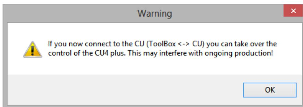
If you now press the button "ToolBox <-> CU" you take over control of the CU and can operate the valves. The text in the status line of the program changes to "ToolBox <-> CU" on yellow background. You can return control to the PLC at any time by pressing the button "PLC <-> CU".
