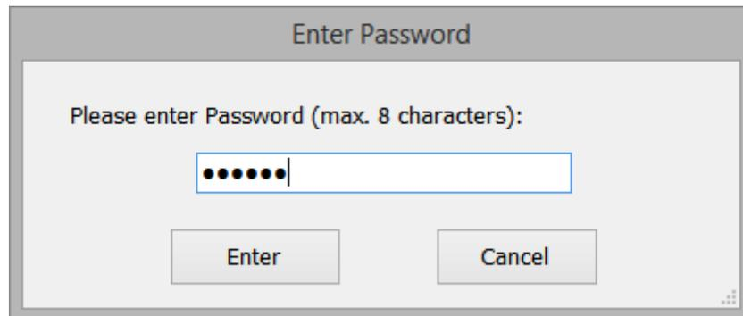
After having entered the correct password the following warning is issued, as now the control of the valve is changed over from the PLC to the Toolbox program.
