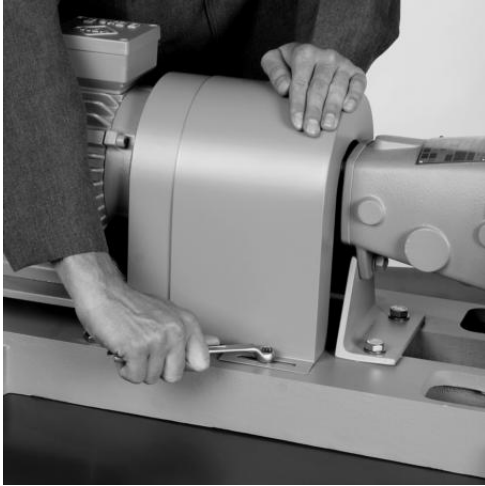
Fig. 7.1 Disconnect electric motor from power supply. Remove safety guard.
