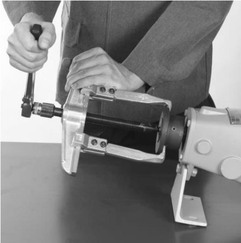
Fig. 7.7 Pull coupling part from shaft end. Loosen safety screw first.
