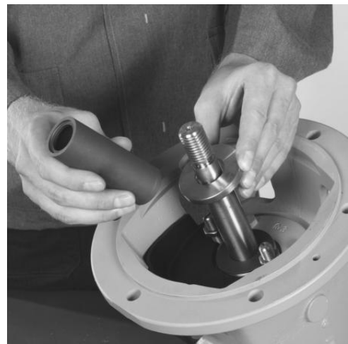
Fig. 7.6 Pull shaft wearing sleeve with O-ring and locking disc system from the shaft.
