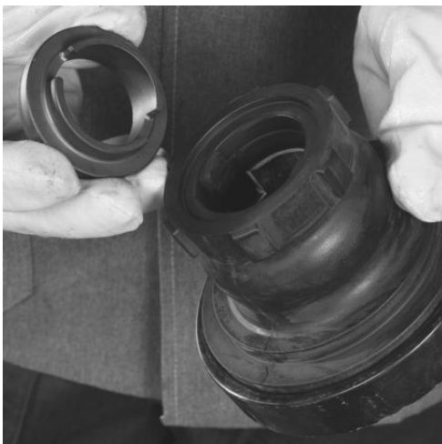
Fig. 7.5 Loosen connection of stationary seal ring, bellows and bellows seat by means of easy pulling.
