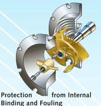
After chopped solids enter the pump, they are prevented from binding the impeller or fouling the seal area by a secondary cutting and clearing action. The impeller's patented rear cutter features a sharpened and serrated rear shroud that sweeps over spiral grooves in the casing back plate. The interaction of the rear cutting shroud and grooves acts to cut and then expel stray material from behind the impeller.
