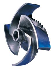
High efficiency, improved NPSH Our patented, computer generated impeller blade profiles provide cutting action at the leading edge while ensuring a smooth flow path for the fluid along the rest of the vane. The smooth flow minimizes turbulence, thereby reducing power consumption and improving NPSH.
