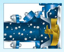
Abrasion Resistant Construction Hayward Gordon's proven clamptype construction eliminates the need for drilled and tapped holes on many wet-end components. This allows construction in a variety of wear resistant metals including Ni-Hard, High Chrome Iron, and hardened alloy steel. To compensate for wear and to maximize component life, clearance between the intake cutting plate and impeller is externally adjustable.
