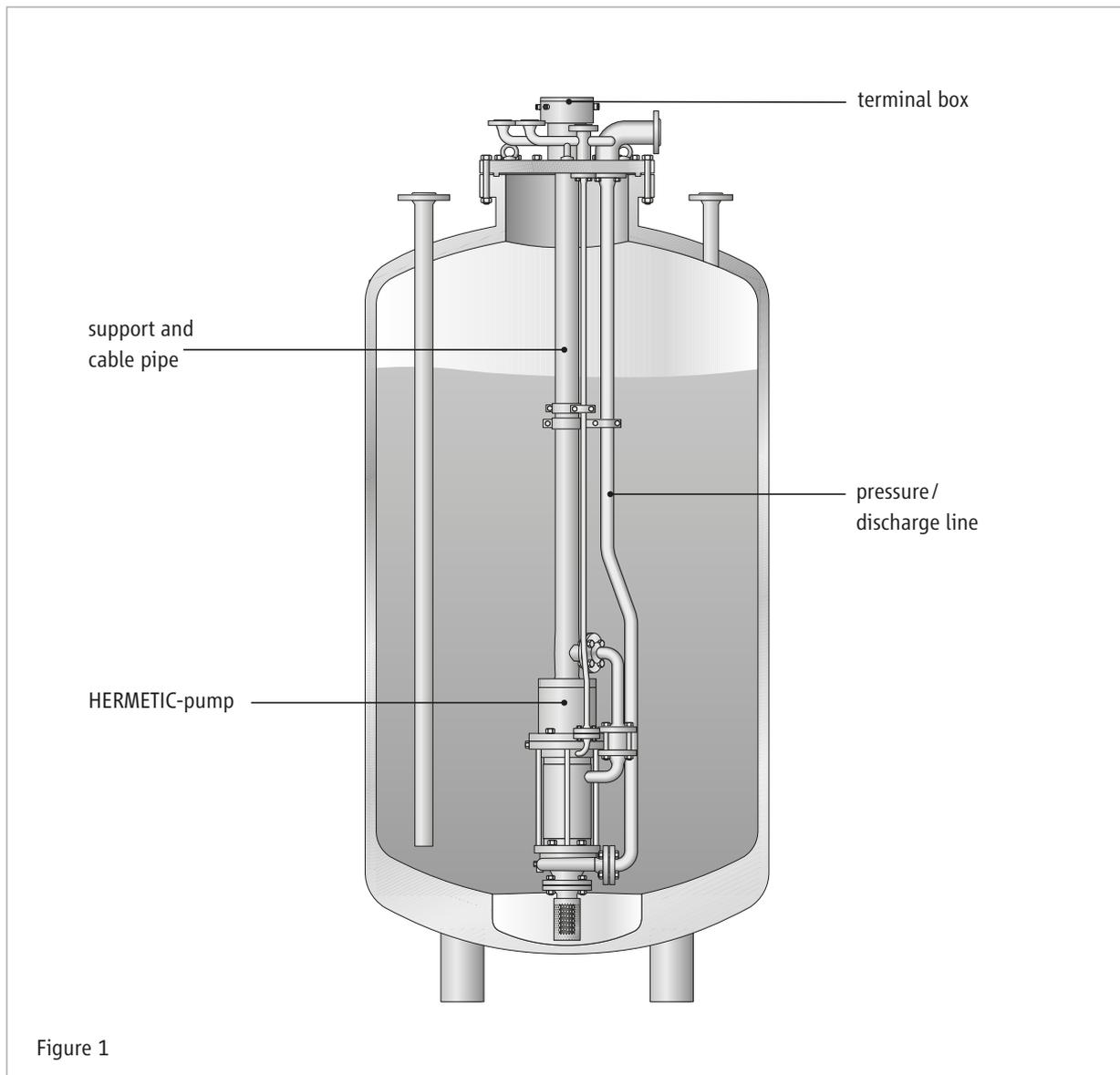
**Installation pump with the opportunity to separate the pump from the liquid in the vessel**
