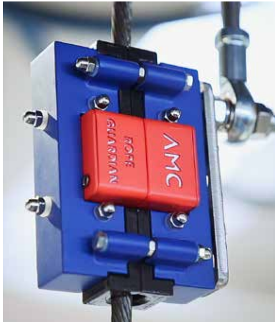
● The AMC devices used for detecting defects inside wire ropes can be either rented or bought.
