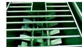
If necessary the pumps can be constructed with wide rectangular inlets to ease the product entry into the pump chamber.
