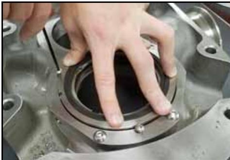
**Figure 120 - Install seal retaining bolts**
