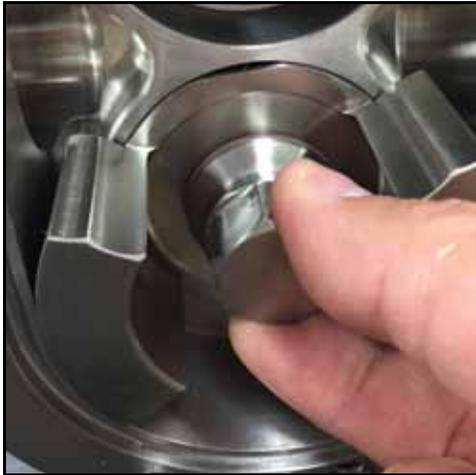
Figure 184 - Install rotor nut
