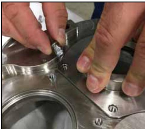
**Figure 61 - Install seal housing bolts**
