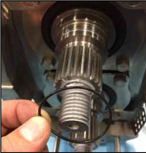
**Figure 122 - Install O-ring**
