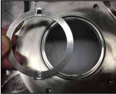
**Figure 86 - Install drive ring**
