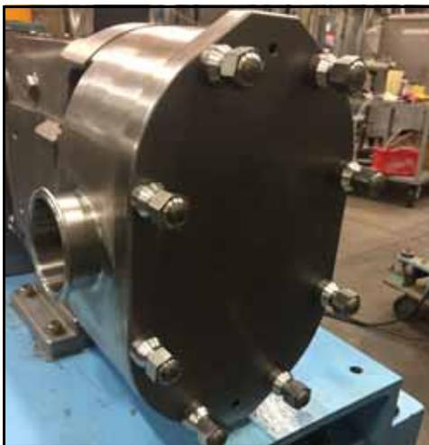
**Figure 191 - Cover installed**
