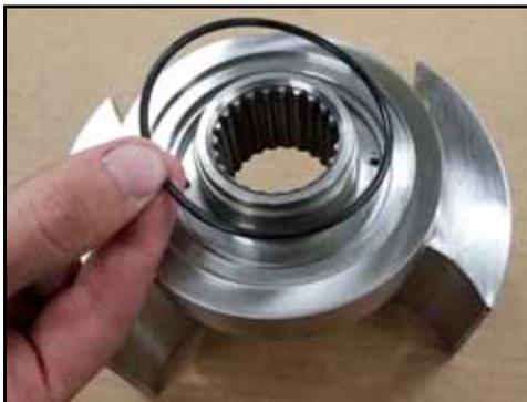
**Figure 172 - Install sleeve front O-ring**
