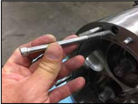
**Figure 170 - Install body retaining screws**
