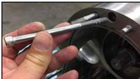
Figure 150 - Remove body retaining screws
