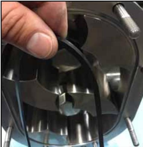
**Figure 187 - Install cover gasket**
