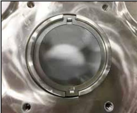
**Figure 57 - drive ring installed (134-U3 and smaller)**
