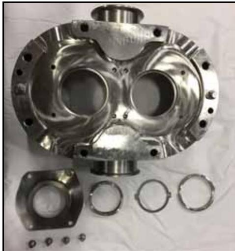
**Figure 53 - Single Mechanical Seal (040-U3 shown)**
