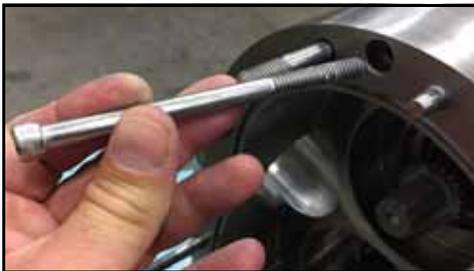
Figure 45 - Remove body retaining screws
