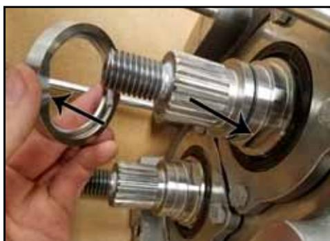
**Figure 165 - Install seal seat**
