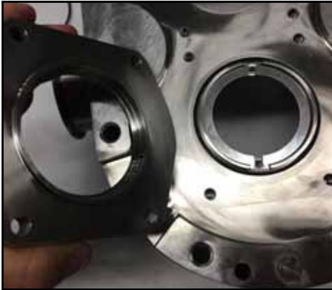
**Figure 90 - Install seal housing**
