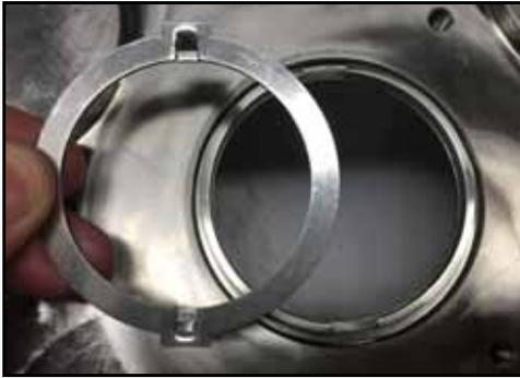
**Figure 56 - Install drive ring**
