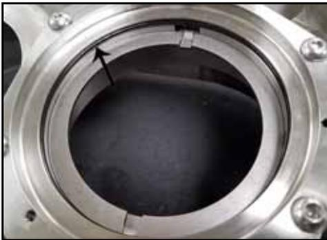
**Figure 117 - Seal O-ring location**
