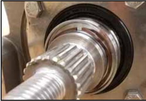
**Figure 167 - Install wave spring**
