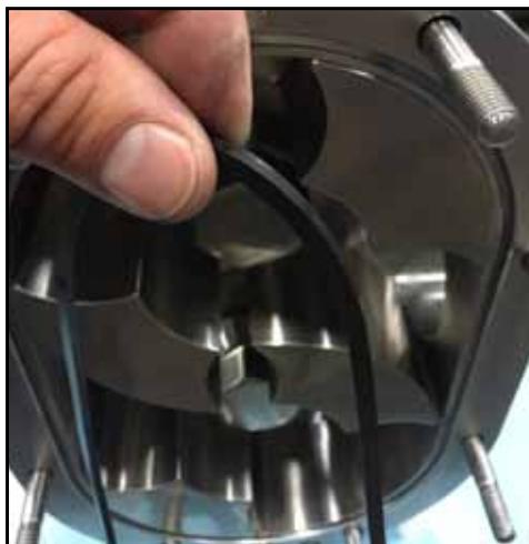
**Figure 37 - Remove cover gasket**
