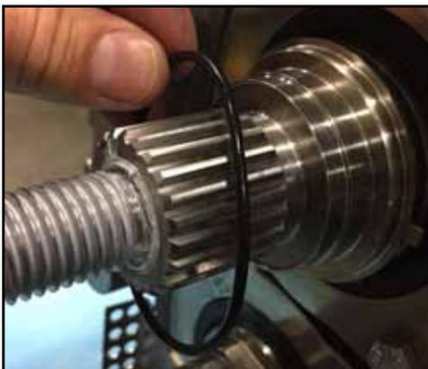
**Figure 106 - Install O-ring**
