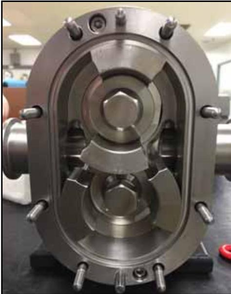
**Figure 186 - Rotors installed**
