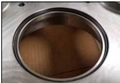
**Figure 158 - Seal housing O-ring installed**
