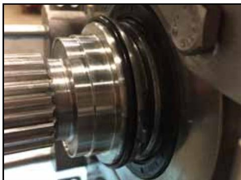
**Figure 127 - O-ring installed**
