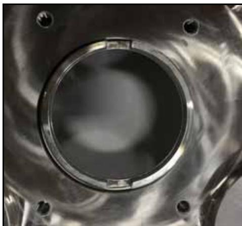
**Figure 55 - Ring installed**
