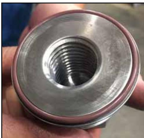
**Figure 183 - O-ring installed**
