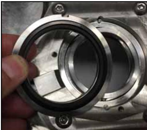
**Figure 74 - Remove stationary seal**
