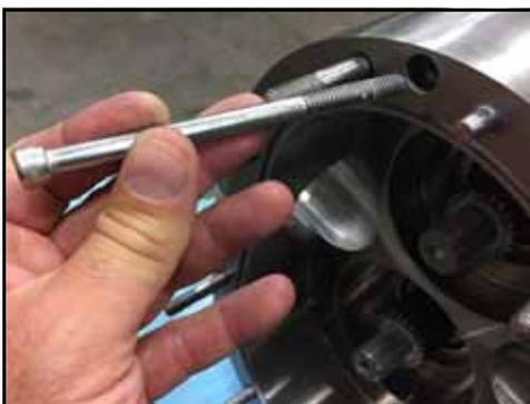
**Figure 132 - Install body retaining screws**
