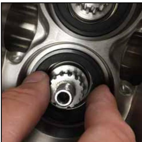
**Figure 136 - Push on stationary seal**
