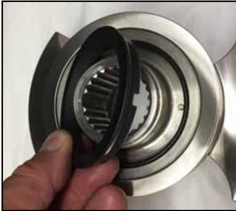
**Figure 140 - Install rotary seal**
