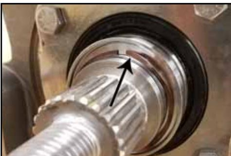
*Figure 155 - Remove wave spring*
