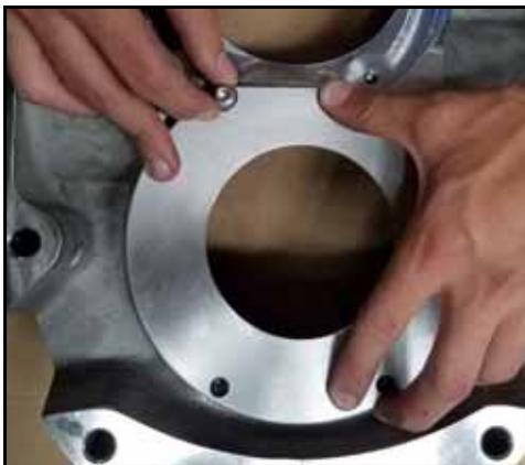
**Figure 67 - Install seal housing bolts**
