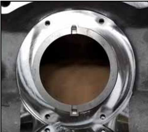
**Figure 64 - Drive ring installed**
