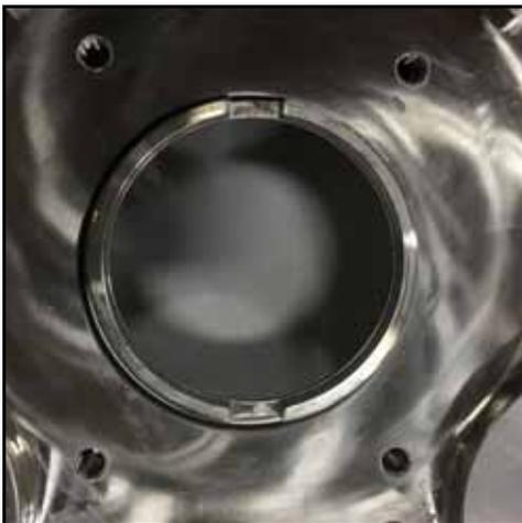
**Figure 85 - Shaft ring installed**
