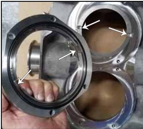
**Figure 113 - Seal housing O-ring installed**
