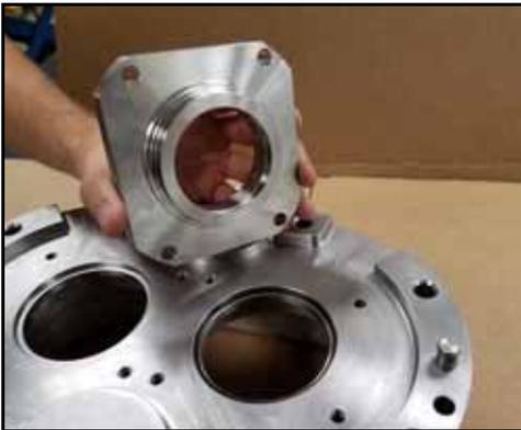
*Figure 153 - Remove seal housing*
