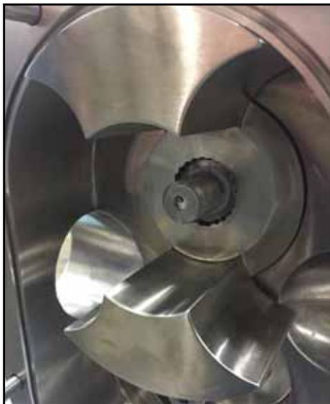
**Figure 181 - Rotor installed**
