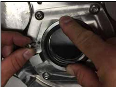
**Figure 99 - Install seal retaining bolts**
