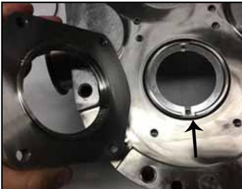
**Figure 78 - Remove seal housing**
