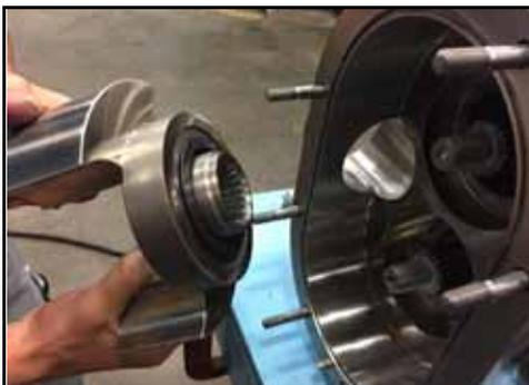
Figure 40 - Remove rotor
