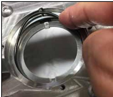
**Figure 93 - Install seal O-ring**
