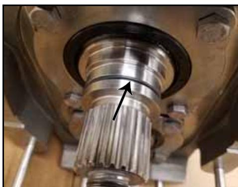
**Figure 164 - O-ring installed**
