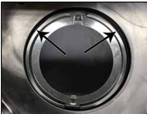
**Figure 89 - Seal housing O-ring installed**
