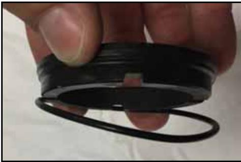
Figure 44 - Stationary Seal O-ring
