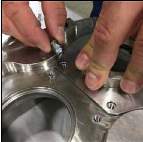
**Figure 47 - Remove seal housing bolts**
