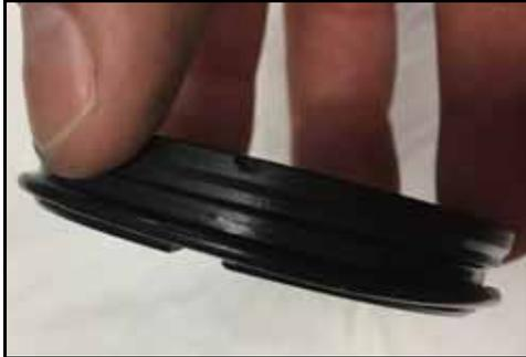
**Figure 134 - Seal O-ring installed**
