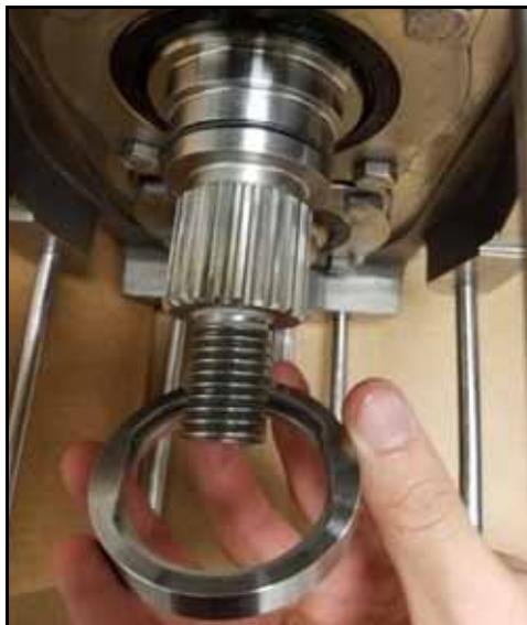
**Figure 156 - Remove seal seat**
