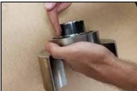
**Figure 177 - Lubricate seal sleeve**
