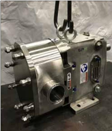
**Figure 3 - Lifting location**
