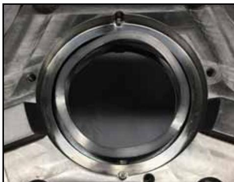
**Figure 96 - Wave spring installed**
