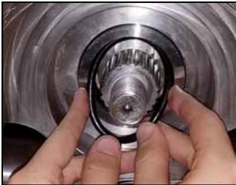
**Figure 171 - Install seal O-ring**
