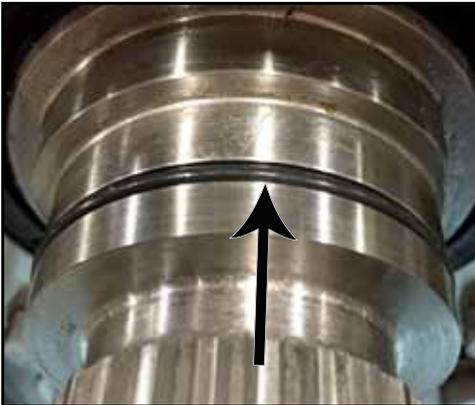
**Figure 123 - O-ring installed**
