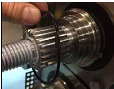
**Figure 126 - Install O-ring**
