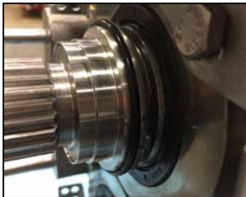
**Figure 107 - O-ring installed**
