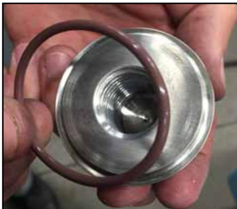
**Figure 182 - Install O-ring**
