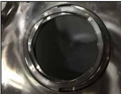
**Figure 59 - Wave spring installed**
