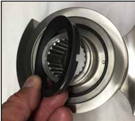
*Figure 41 - Remove rotary seal*
