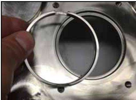
**Figure 82 - Remove shaft ring**
