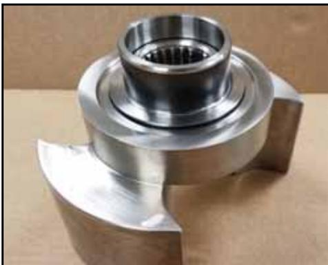
**Figure 176 - Seal sleeve installed**
