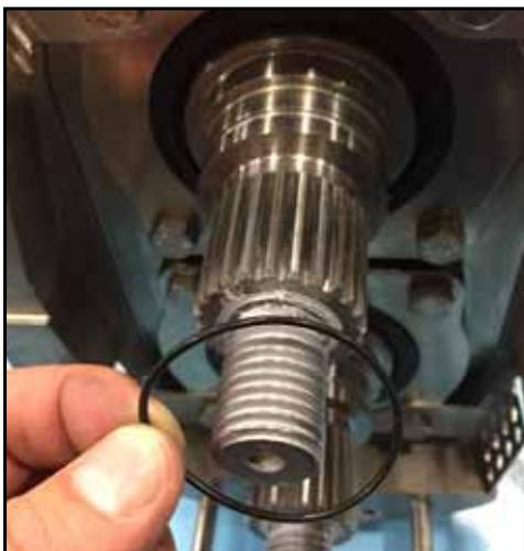
**Figure 102 - Install O-ring**
