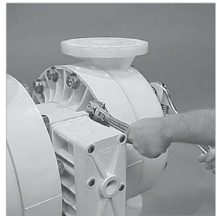
Step 4 Remove air valve end cap to expose air valve spool by simply lifting up on end cap once air valve bolts are removed
