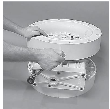
Step 1 Loosen the air valve bolts utilizing a 3/8" hex-head wrench.
