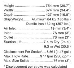
at 4.8 bar (70 psig) air inlet pressure against a 2 bar (30 psig) head pressure.
