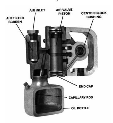
The air valve assembly consists of both the air valve body and piston and the center block. The unique design of the air valve relies on differential pressure to effect the diaphragm shift. It is reliable and simple to maintain. The bushing in the center block, along with the diaphragm shaft, provides the "trigger" to tell the air valve to shift. The following procedure will ensure that the air valve on your Wilden pump will provide long-lasting trouble-free service.
