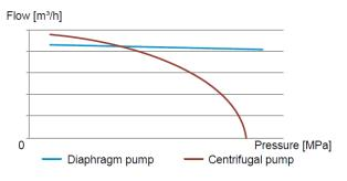
Flow vs. pressure operating curve
