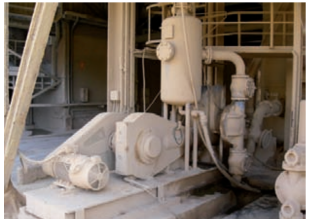
60 m 3 /h (260 GPM); 1.0 MPa (145 psi), Medium: sulphate slurry, solids concentration: 50%, density: 1.6 kg/ up to 8 mm particle size.
