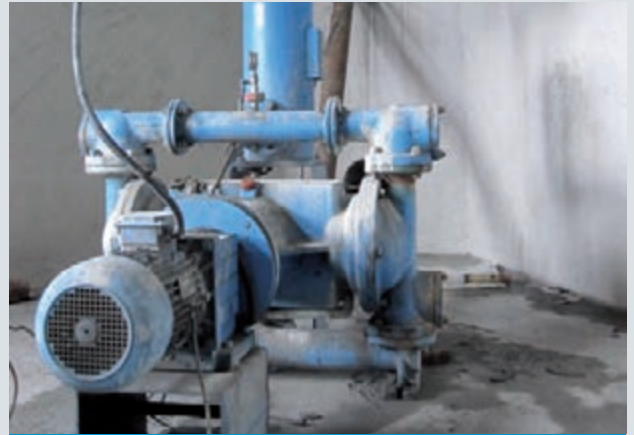
ABEL EM-080 for transfer of thickened ore tailings
