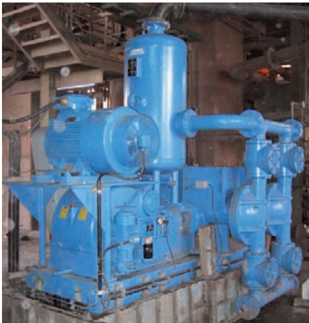
100 m 3 /h (440 GPM); 1.6 MPa (225 psi), Medium: iron ore tailings, solids concentration: 47 %, up to 3 mm particle size.
