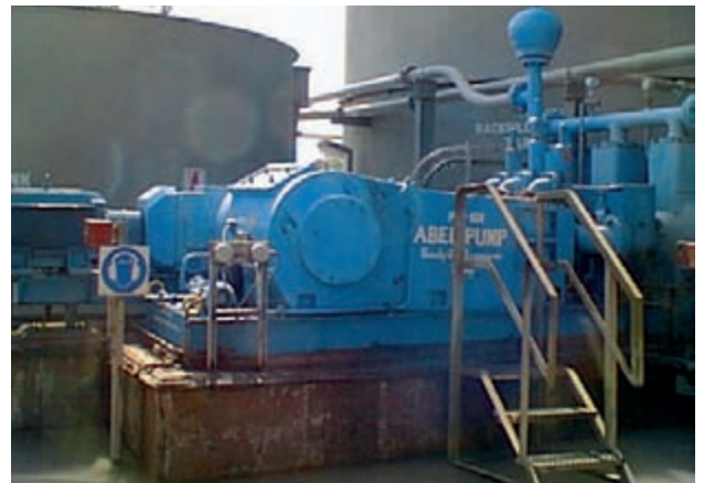
Classified copper tailings, 50% solids concentration. 90 m 3 /h (390 gpm); 50.0 MPa (720 psi). Transfer distance: 3.5 km (2.2 miles).
