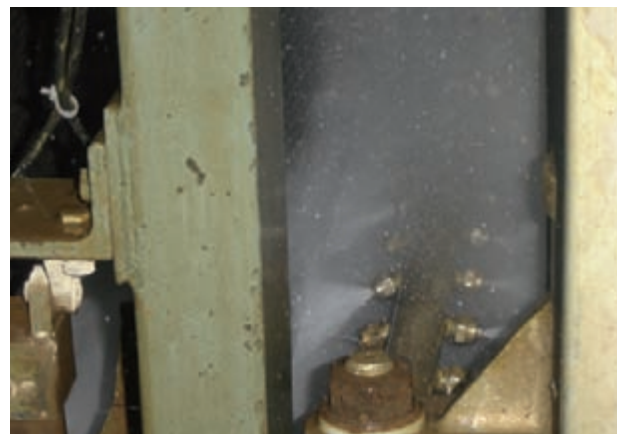
Jet arm of a washing device for filter cloth cleaning
