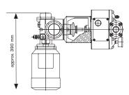
Weight, according to equipment (without motor) approx. 19-106 kg
