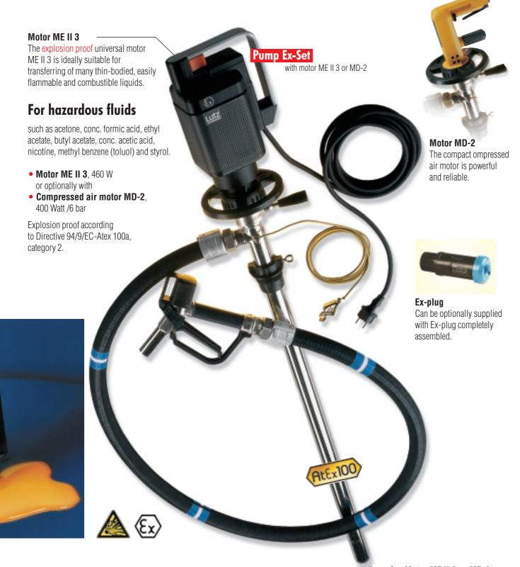
Pump Set: **Motor ME II 3 or MD-2**, **pump tube RE-SS 41-L-MS** stainless steel, **2,5 m** universal chemical hose 1", electrically conductive bound with hose connectors stainless steel, nozzle stainless steel (1.4571), equipotential bonding cable, drum adapter PP (without Ex-plug)
