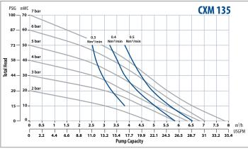
The data refers to water (20°C, 68°F), under use of different pump variations, a compressor Atlas Copco VSG30 and calibrated measuring equipment.
