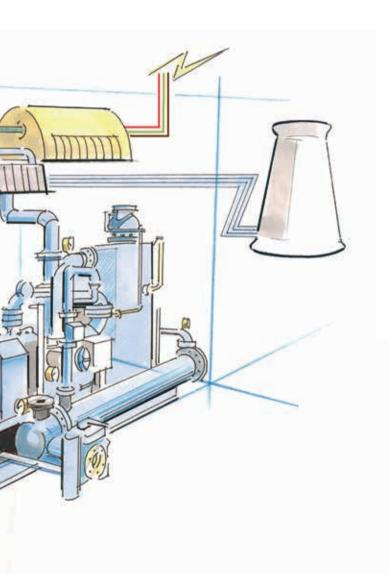
The vacuum pump system is comprised of a single stage liquid ring pump complete with a total seal water recirculation system, sized to meet the process duty requirements. If duty and standby pumpsets are called for, then two systems are provided, giving true standby capability including the seal water recirculation system.
