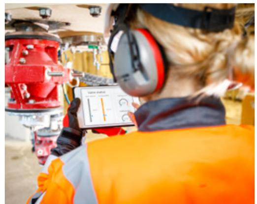
*The Flowrox smart instrumentation can be retrofitted to automatic pinch valves.*
