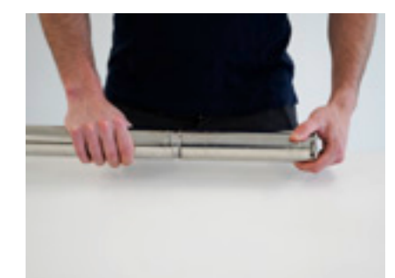
Unscrew stator housing
