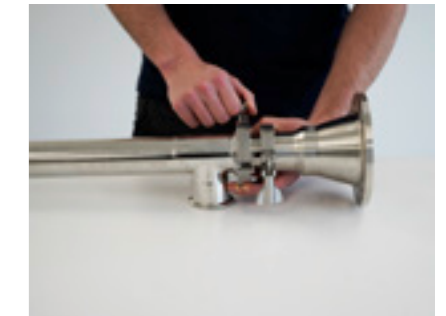
Open clamp on pump tube
