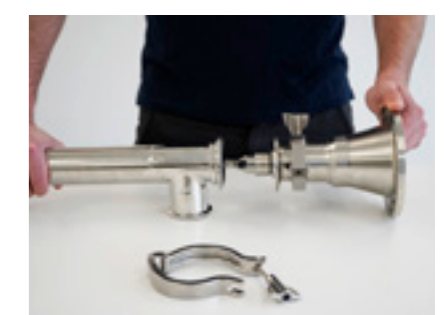
Remove pump tube
