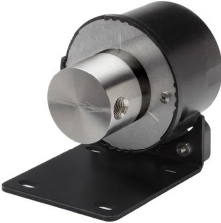
When you need a low-flow pump that delivers high performance in a small package, Series GA is an excellent option. Series GA gear pumps provide precise, pulseless flow, and features Micropump's suction shoe design. The suction shoe self-compensates for wear, ensuring near zero slip and long pump life. This pump, standard with an electromagnetic EagleDrive™, provides a highly efficient, compact pumping package that easily integrates into your design.
