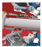
M2 MG12 / M7N single mechanical seal unbalanced
