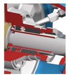
\$3 stuffing box with shaft sleeve and lantern ring
