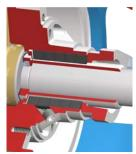
**\$2** stuffing box with shaft sleeve
