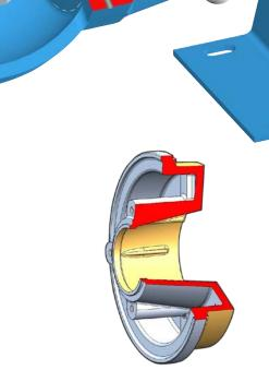
tapered bore seal chamber option
