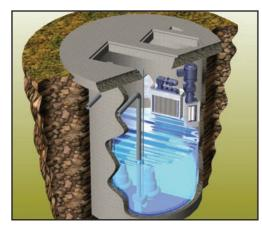
Discreen / Muncher combination for pump protection
