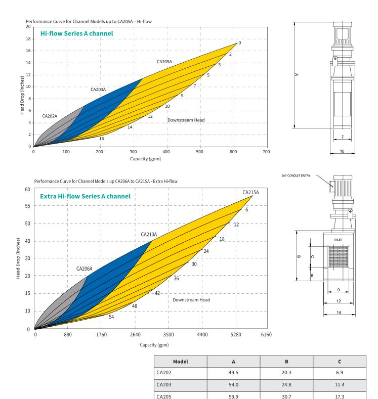
All dimensions are in inches and for guidance only. For more information about the Series A Muncher, contact NOV.
