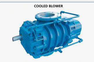
The blower is equipped with two cooling coils that keep the oil temperature below 100°C in all operating conditions. This version is recommended when the gas discharge temperature exceeds 140°C.
