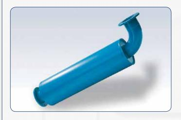
To be fitted on ROBOX evolution units for vacuum operation: ES../V and ES../DV. Consisting of SDL absorption silencers and SPS exhaust silencers. This reduces the sound pressure level generated by the exhaust outlet by approximately 25 dB(A) within the frequency field ranging from 200 Hz to 20 kHz.
