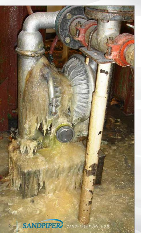
breached, the fluid enters the air distribution system and escapes into the environment through the muffler, requiring immediate service. This results in:
