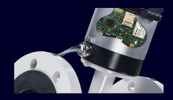
The 4G-based IIoT Wireless Communication Module collects measurement data from meters anywhere in the world covered by a LTE-M, NB-IoT or 2G network. Measurement data, parameters and alarms from the MAG 8000 are made accesible via the IIoT Web Application.
