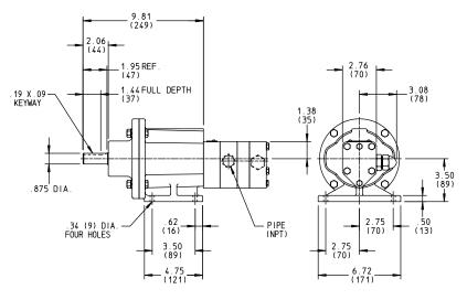
Dimensions for Viking SG Sealless Mag Drive Series Motor Mount - MD-A\_B Drive Sizes - SG-807 & SGN-807
