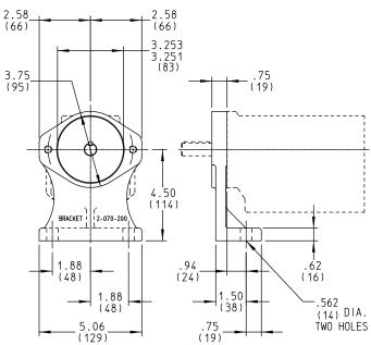
Note: Shaft height corresponds to Viking's "A" reducer or NEMA 56, 143T and 145T motors.
