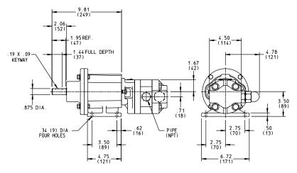
Dimensions for Viking SG Sealless Mag Drive Series Motor Mount - MD-B\_B Drive Sizes - SG-807 & SGN-807
