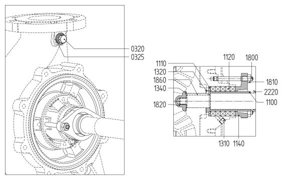
Figure 53: Stuffing box packing S2.
