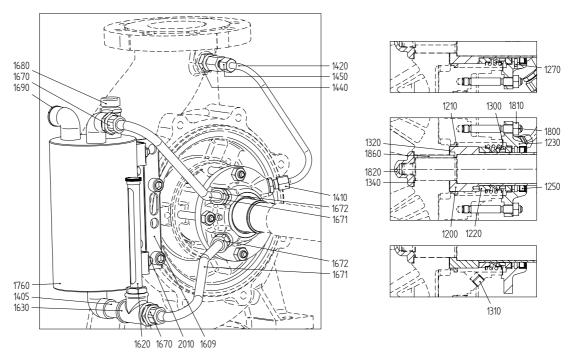
Figure 24: Mechanical seal MQ...
