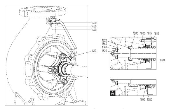
Figure 79: Mechanical seal C2 - UNITEX (A = br.gr 2 and 3).
