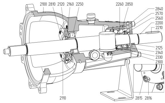
Figure 32: Bearing L6 (reinforced, oil-lubricated, adjustable).
