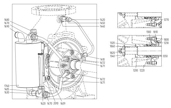
Figure 73: Mechanical seal MQ3 - HJ92N.
