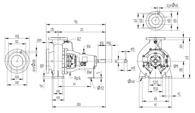
Figure 36: Pump dimensions - bearing groups 0, 1, 2, 3.
