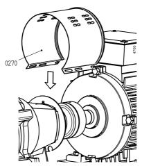
Figure 13: Fitting the jacket at motor side.
