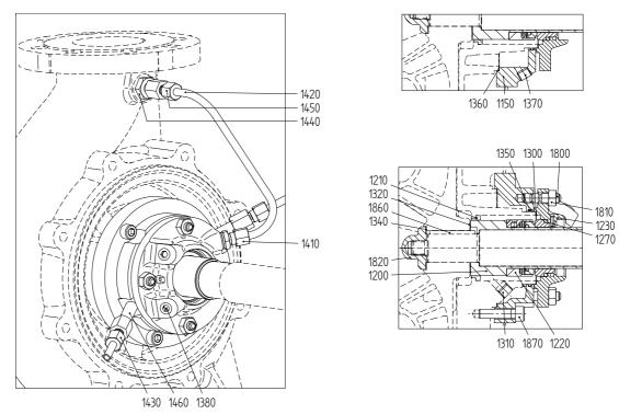
Figure 74: Mechanical seal MW2 - M7N.
