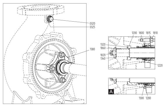
Figure 78: Mechanical seal C2 - UNITEX (A = br.gr 2 and 3).
