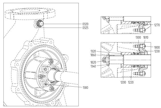
Figure 63: Mechanical seal HJ92N.
