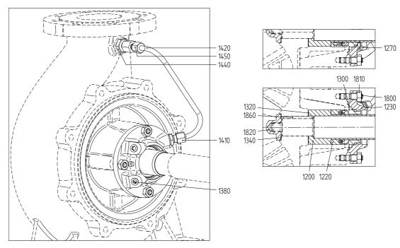
Figure 60: Mechanical seal M7N.
