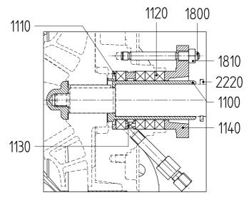
Figure 22: Stuffing box packing S2, S3 and S4.
