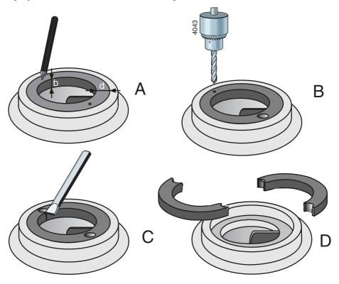
Figure 19: Removal of wear ring.
