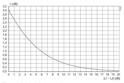
Figure 99: Noise level of entire pump unit.
