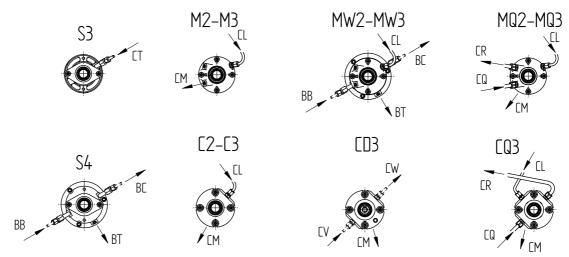
Figure 35: Connections for bearing groups 0, 1, 2, 3.
