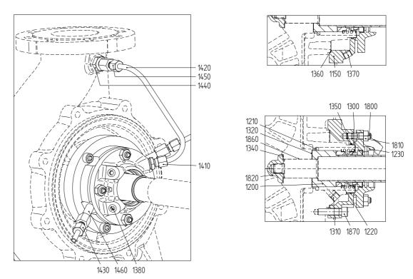
Figure 75: Mechanical seal MW2 - MG12-G60.
