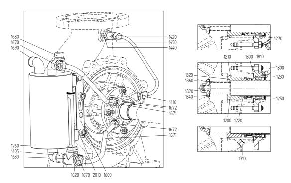
Figure 71: Mechanical seal MQ3 - HJ92N.
