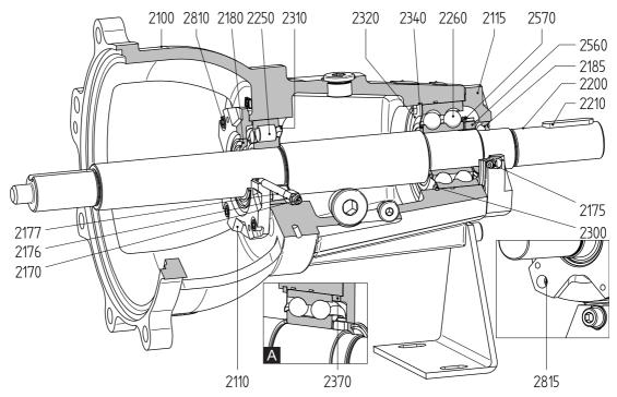
Figure 29: Bearing L2 (reinforced, grease-lubricated) (A = bearing group 3).
