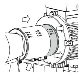
Figure 17: Adjusting the jacket at motor side.
