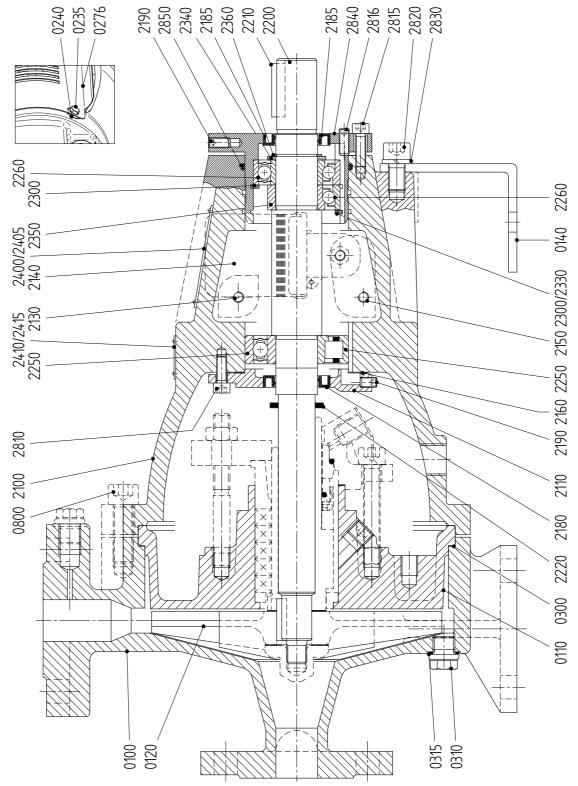
Figure 52: Sectional drawing L5 / L6 - 25-....
