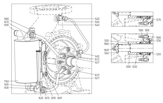
Figure 69: Mechanical seal MQ2 - M7N.
