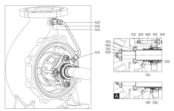
Figure 77: Mechanical seal C2 - UNITEX (A = br.gr 2 and 3).
