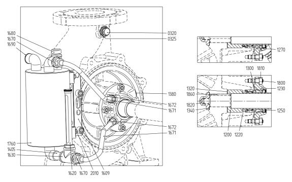
Figure 72: Mechanical seal MQ3 - HJ92N.
