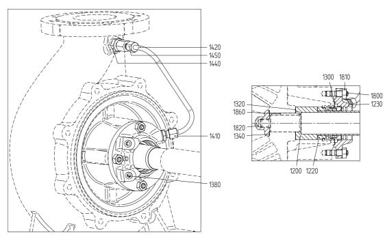
Figure 61: Mechanical seal MG12-G60.
