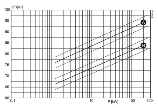
Figure 98: Noise level as function of pump power [kW] at 2900 min<sup>-1</sup> A =sound power level, B =sound pressure level.
