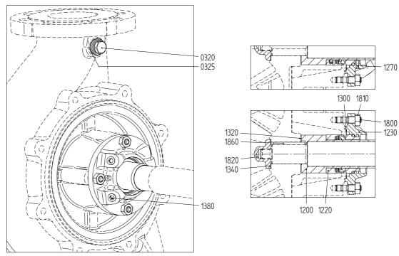
Figure 58: Mechanical seal M7N.
