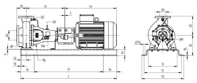
Figure 37: Pump-motor unit - bearing groups 0, 1, 2, 3 - with standard coupling.
