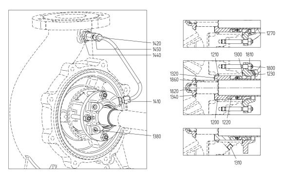
Figure 23: Mechanical seal M2-M3.
