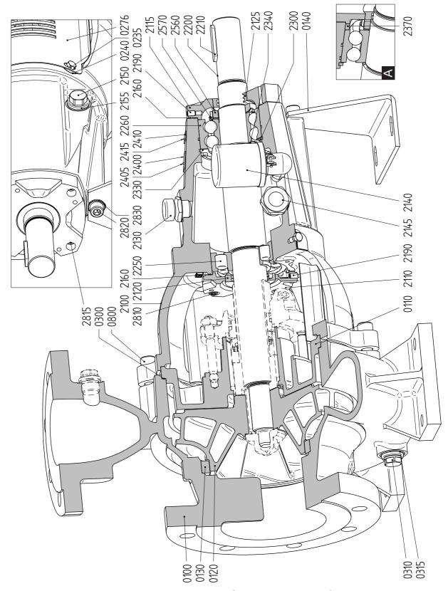
Figure 46: Sectional drawing L4 (A = for bearing group 3).
