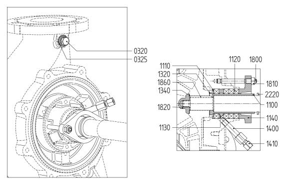
Figure 54: Stuffing box packing S3.
