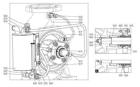
Figure 85: Mechanical seal CQ3 - CARTEX QN (A = br.gr. 3).
