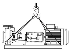
Figure 1: Lifting instructions for pump unit.
