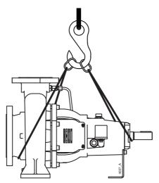
Figure 2: Lifting instructions for single pump.
