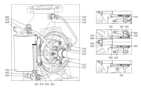
Figure 65: Mechanical seal MQ2 - M7N.
