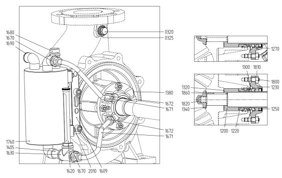
Figure 68: Mechanical seal MQ2 - MG12-G60.
