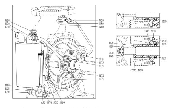
Figure 70: Mechanical seal MQ2 - MG12-G60.
