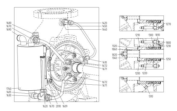
Figure 66: Mechanical seal MQ2 - MG12-G60.
