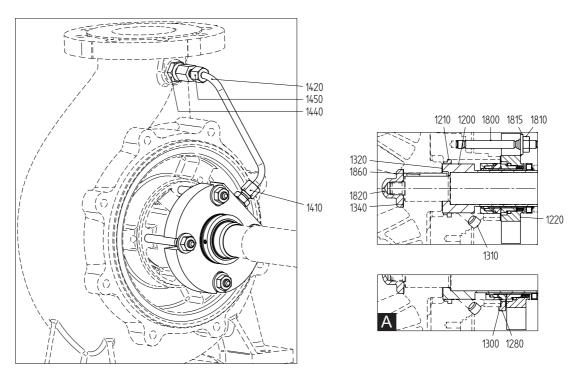
Figure 80: Mechanical seal C3 - CARTEX SN (A = br.gr. 3).
