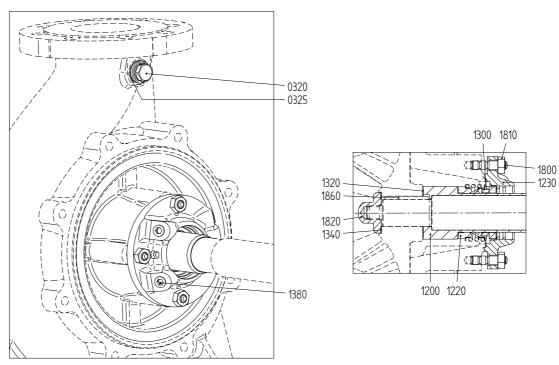
Figure 59: Mechanical seal MG12-G60.
