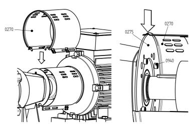
Figure 16: Fitting the jacket at pump side.
