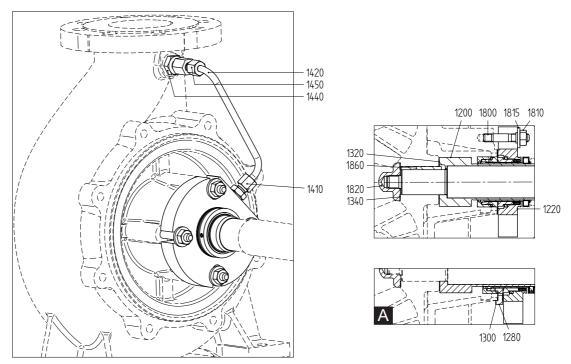
Figure 82: Mechanical seal C3 - CARTEX SN (A = br.gr. 3).
