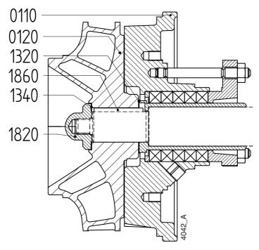
Figure 18: Disassembling the impeller.
