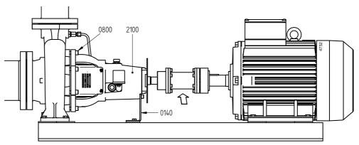
Figure 12: Back-Pull-Out principle.
