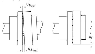
Figure 9: Alignment tolerances standard coupling.
