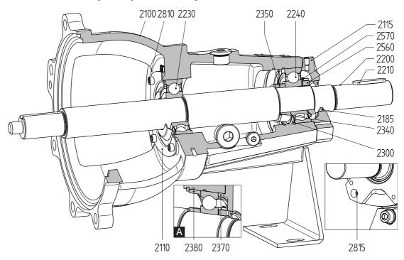
Figure 27: Bearing L1 (standard, grease-lubricated) (A = bearing group 3).
