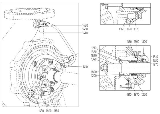
Figure 76: Mechanical seal MW3 - HJ92N.
