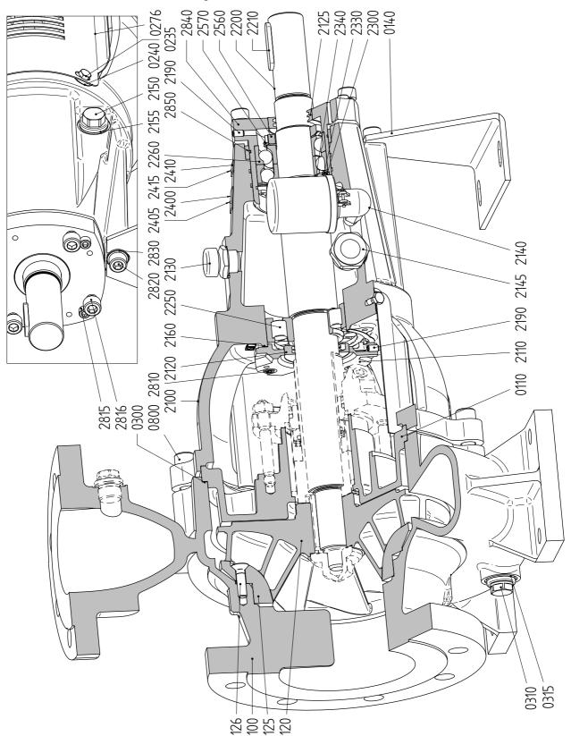
Figure 50: Sectional drawing L6.
