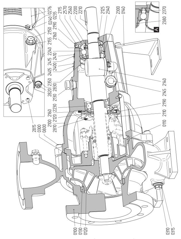
Figure 44: Sectional drawing L3 (A = for bearing group 3).
