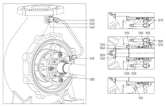
Figure 62: Mechanical seal HJ92N.
