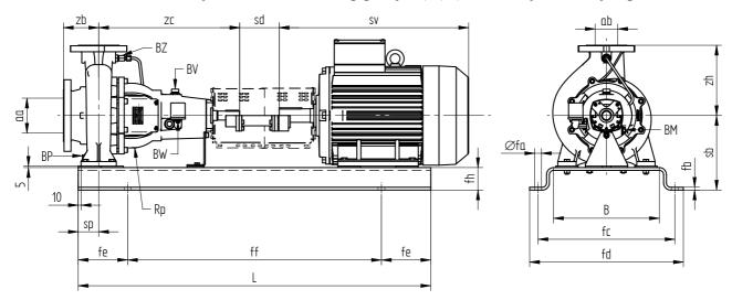
Figure 38: Pump-motor unit - bearing groups 0, 1, 2, 3 - with spacer coupling.
