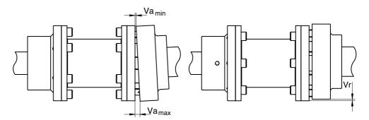
figure 10: Alignment tolerances spacer coupling.
