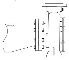
Figure 11: Eccentric reducer to suction flange.
