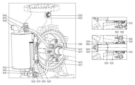
Figure 67: Mechanical seal MQ2 - M7N.
