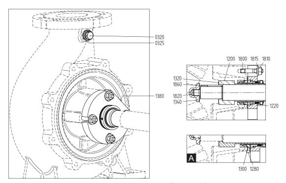
Figure 81: Mechanical seal C3 - CARTEX SN (A = br.gr. 3).
