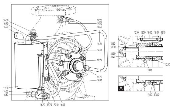
Figure 83: Mechanical seal CQ3 - CARTEX QN (A = br.gr. 3).
