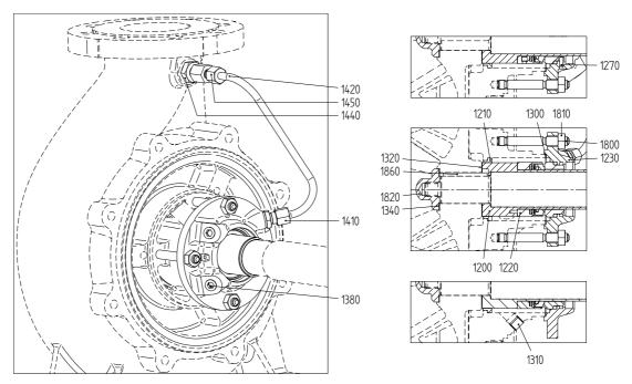
Figure 56: Mechanical seal M7N.
