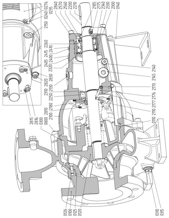
Figure 49: Sectional drawing L5 with tapered bore.
