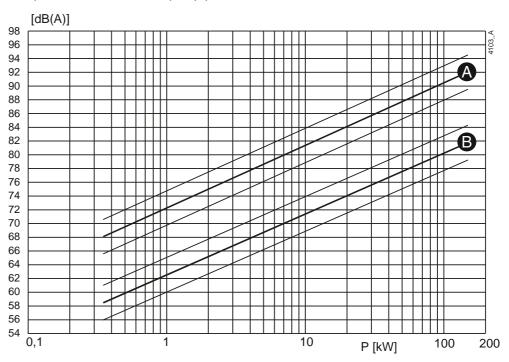
Figure 97: Noise level as function of pump power [kW] at 1450 min<sup>-1</sup> A = sound power level, B = sound pressure level.
