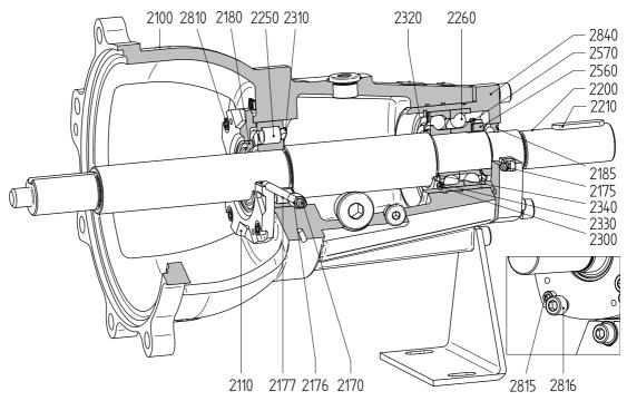
Figure 31: Bearing L5 (reinforced, grease-lubricated, adjustable).
