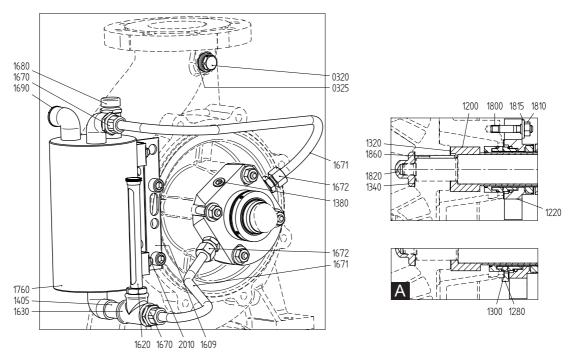
Figure 84: Mechanical seal CQ3 - CARTEX QN (A = br.gr. 3).
