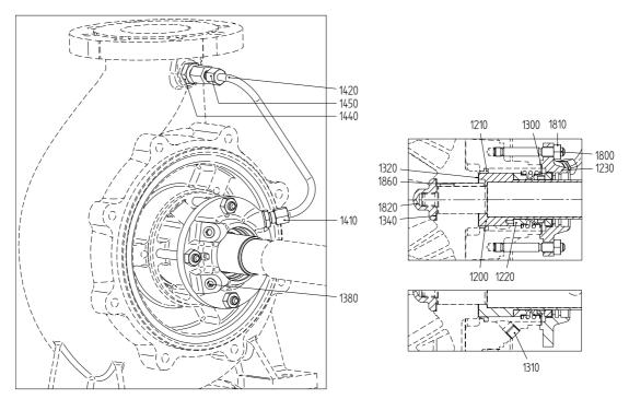
Figure 57: Mechanical seal MG12-G60.
