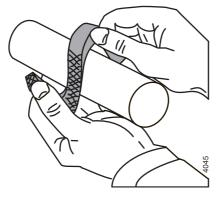
Figure 21: Axially bending open packing rings.
