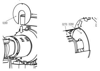
Figure 14: Fitting the assembly plate at motor side.
