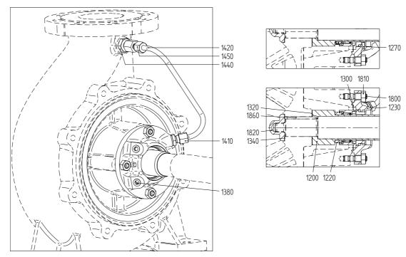
Figure 64: Mechanical seal HJ92N.
