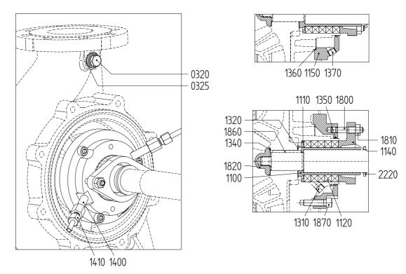
Figure 55: Stuffing box packing S4.
