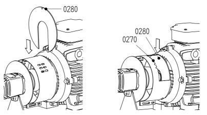
Figure 9: Fitting the assembly plate at motor side.
