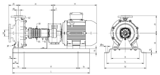
*Figure 18: Pump-motor unit with standard coupling.*
