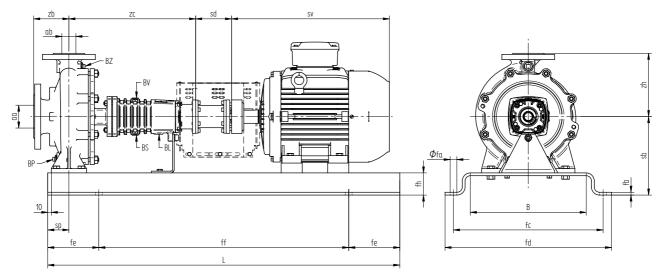
*Figure 19: Pump-motor unit with spacer coupling.*
