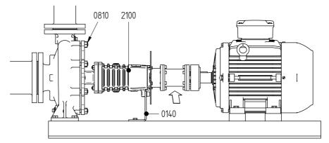
Figure 7: Back-Pull-Out principle.
