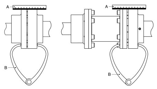
Figure 3: Aligning the coupling by means of a ruler and a pair of outside calipers.
