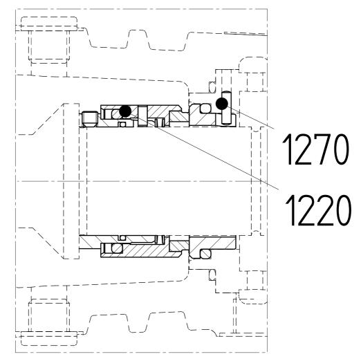
Figure 23: Mechanical seal HJ92N.
