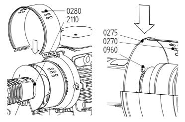
Figure 11: Fitting the jacket at pump side.
