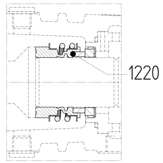
Figure 22: Mechanical seal MG12-G60.
