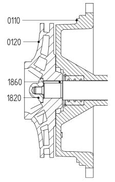
*Figure 13: Disassembling the impeller.*
