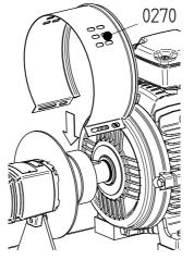
Figure 8: Fitting the jacket at motor side.
