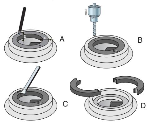
Figure 14: Removal of wear ring.
