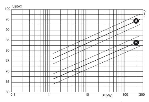
Figure 31: Noise level as function of pump power [kW] at 2900 min<sup>-1</sup> A = sound power level, B = sound pressure level.
