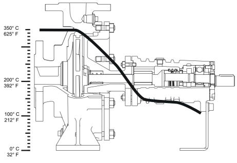
Figure 24: Temperature dissapation in the pump.
