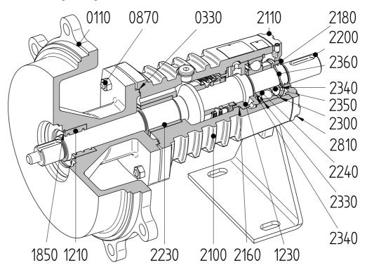
Figure 15: Bearing L1 and mechanical seal M1, M5).
