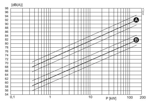
*Figure 30:* Noise level as function of pump power [kW] at 1450 min<sup>-1</sup> A = sound power level, B = sound pressure level.
