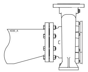
Figure 6: Eccentric reducer to suction flange.
