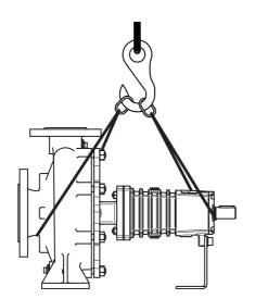
*Figure 2: Lifting instructions for single pump.*
