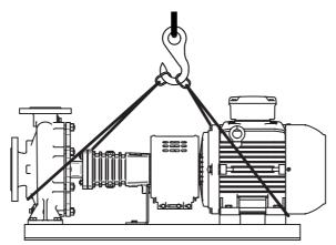
Figure 1: Lifting instructions for pump unit.
