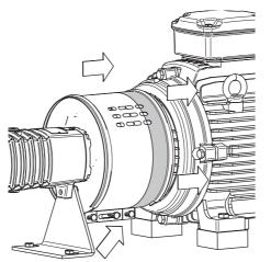
Figure 12: Adjusting the jacket at motor side.
