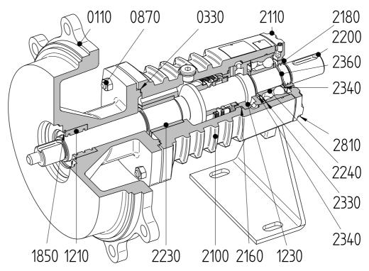
Figure 16: Bearing L2 and mechanical seal M1, M5).
