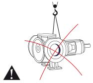
Never lift the pump unit with only two fastening points. Incorrect lift can cause personal injury and/or damage to the pump unit.
