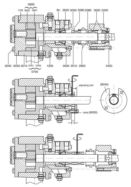
Assembly of a double mechanical seal "back-to-back" (GD)
