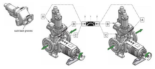
When a double safety relief valve is installed three arrow plates are attached – one on each valve (A and B) indicating the liquid flow direction of each valve (small arrows 2 and 3) and one on the Y-casing (C) indicating the most favourable direction of rotation of the pump (arrow 1).
