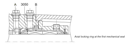
This locking ring prevents the static part of the mechanical seal from being pushed out of its seat in case quench pressure (B) falls back or drops out.
