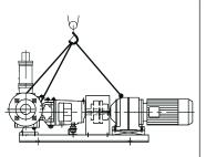
If there are lifting rings on both the pump and the motor the slings may be fastened to these.
