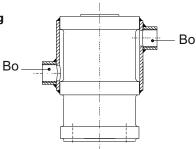
In case of steam supply, connect the supply line at the highest position and the return line to the lowest position so that condensed water will be drained via the lowest line. In case of liquid supply, the positions are not important.
