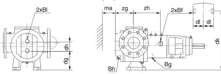
Jackets (TT) with flange connections on pump cover and around shaft seal
