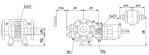
Single jacket (SO) with thread connection on pump cover Single jacket (TO) with flange connection on pump cover
