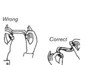
Bending and twisting packing rings
