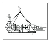
Secure lifting slings around the front part of the pump and the back part of the motor. Make sure that the load is balanced before attempting the lift.
