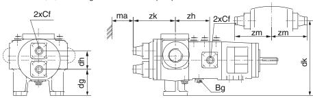
Single jacket (SO) with thread connection on pump cover Single jacket (TO) with flange connection on pump cover
