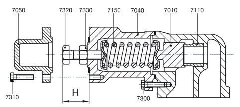
Assembly and disassembly of the safety relief valve
