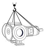
Always use two or more lifting slings. Make sure they are secured in such a way as to prevent them from slipping. The pump unit should be in a straight fashion.
