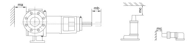
It is imperative that the operating device of pump and/or pump unit is always accessible (also during operation).
