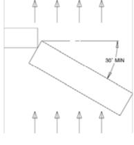
Figure 5 Minimum installation angle
