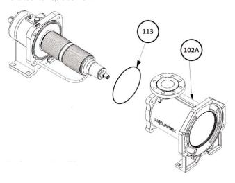
Assembly is undertaken in the reverse order of dismantling, taking care to correctly position the seal 113 and the indexing pins 117 and 513. The screws 147 must be remounted with thread locking adhesive (Loctite® 243\* or equivalent): 4 x M16: Assembly torque 90 Nm.
