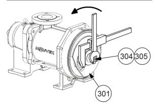
To make handling of the cylinder/piston unit easier, move the lifting ring from the transmission body to the cylinder.
