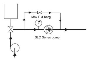
It is preferable not to run the SLC Series pump during CIP, although low speed (< 100 rpm) is acceptable by alternating start/stop operation.
