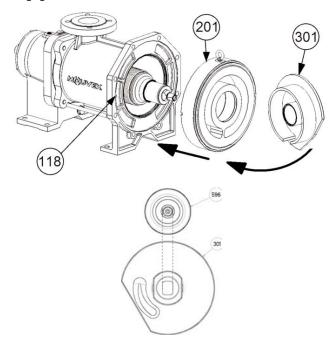
Place thread locking adhesive (Loctite® 243\* or equivalent) on the thread of the transmission hub 596.
