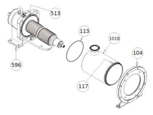
Assembly is undertaken in the reverse order of dismantling, taking care to correctly position the seal 113 and the indexing pins 117 and 513. The nuts 115 must be re-mounted with thread locking adhesive (Loctite® 243\* or equivalent):
