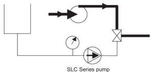
The SLC Series pump is stopped when cleaning the installation.
