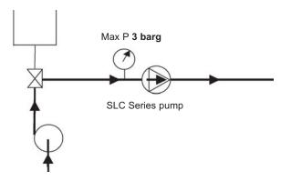
It is preferable not to run the SLC Series pump during CIP although low speed (< 100 rpm) is acceptable by alternating start/stop operation.
