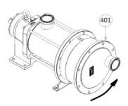
• Remove the outlet tube 402 and its seals 205.
