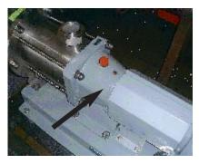
When looking at the shaft, the rotation will be clockwise. When looking at the front cover, the direction of rotation will be anti-clockwise.
