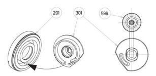
Place thread locking adhesive (Loctite® 243\* or equivalent) on the thread of the transmission hub 596.
