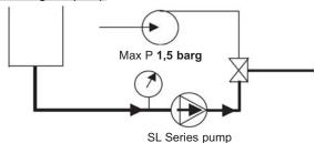
We recommend limiting the rotation speed of the SL Series pump.
