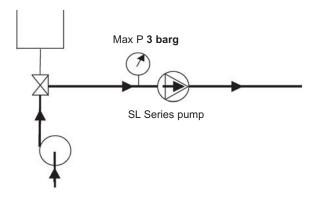
It is preferable not to run the SL Series pump during CIP although low speed (< 100 rpm) is acceptable by alternating start/stop operation.
