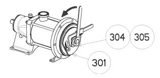
• With the help of a hub puller, extract the piston 301.
