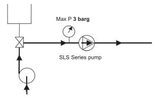
It is preferable not to run the SLS Series pump during CIP although low speed (< 100 rpm) is acceptable by alternating start/stop operation.
