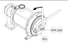
To make handling of the cylinder/piston unit easier, move the lifting ring from the transmission body to the cylinder.
