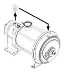
Screw the lifting hook in the tapped hole of the cylinder, provided for this purpose and tighten the screw in the location of the lifting ring.
