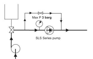
It is preferable not to run the SLS Series pump during CIP, although low speed (< 100 rpm) is acceptable by alternating start/stop operation.
