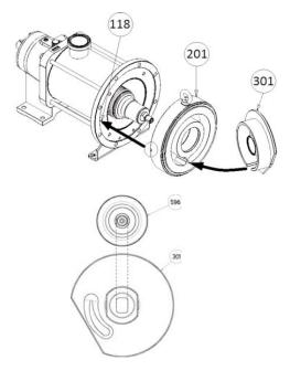
• Place thread locking adhesive (Loctite<sup>®</sup> 243\* or equivalent) on the thread of the transmission hub **596**.
