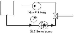
We recommend limiting the rotation speed of the SLS Series pump.
