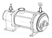
• With the help of a hub puller, extract the piston **301**.
