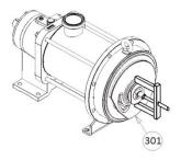
• Remove the cylinder 201 and the seals 113 and 306.
