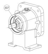
Re-mount the cover 607 after placing the seal 602, greasing the lips of the seals and greasing between the 2 seals 608.
