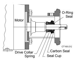
Figure 31 - Installing Seal
