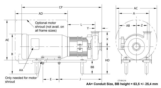
Figure 3 - Pump Dimensions with IEC Motor with optional motor shroud
