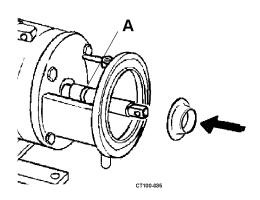
Figure 24 - Installing Deflector
