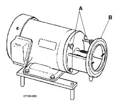
Figure 20 - Removing the Adapter
