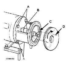
Figure 22 - Adapter Installation
