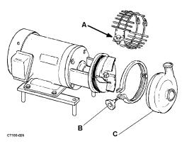
Figure 14 - Casing Assembly
