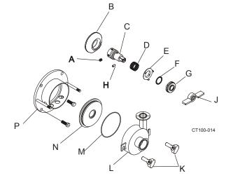
Figure 2 - Pump Components for C-100
