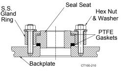
Figure 29 - Stationary Seal Seat
