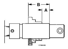
Figure 25 -Drive Collar for "D" Seal Type Adjustment
