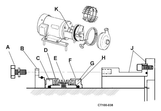
Figure 35 - Parts Stack for Stuffing Box
