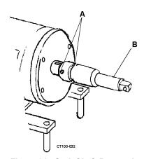
Figure 21 - Stub Shaft Removal
