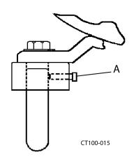
Figure 4 - Leveling Leg Setscrew Location
