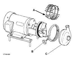
Figure 28 - Casing Clamp Guard Assembly
