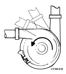
Figure 6 - Recommended Discharge Positions
