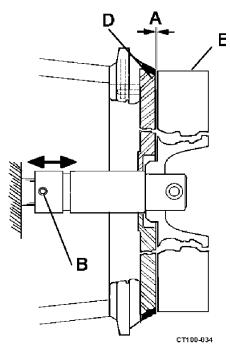
Figure 23 - Setting Backplate/Impeller Clearance
