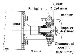
Figure 32 - Installing backplate and impeller
