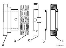
Figure 26 - Carbon Seal
