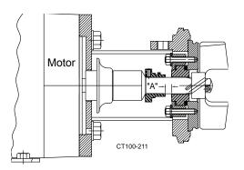
Figure 30 - Drive Collar Adjustment for "DG" Seal
