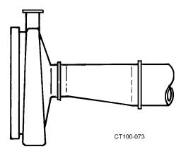
Figure 8 - Correct Eccentric Installation
