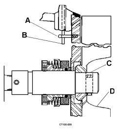
Figure 27 - Backplate Installation
