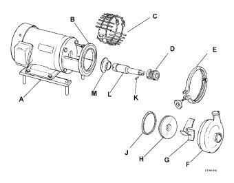
Figure 1 - Pump Components for C-114 through C-328
