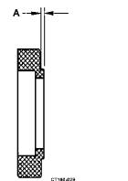
Figure 18 - Carbon Seal Measurements
