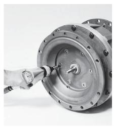
**Step 4**Using a 5/16" hex-head wrench, remove the air chamber fasteners.
