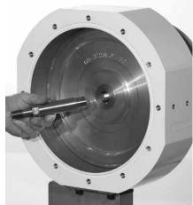
Step 28 Remove the outler piston, diaphragm and shaft assembly from the air chamber.
