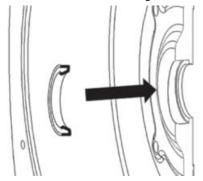
If necessary to replace friction ring 27, use a mallet and a chisel, to break and remove friction ring 27.
