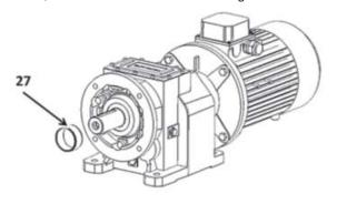
Heat new friction ring at 110 ±10°C / 230 ±50°F.
