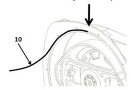
$\underline{\text{Incorrect mounting}}$  : risk of leak and body vacuuming impossible.
