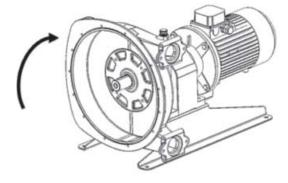
Refit rotor in the pump (see § ROTOR REMOVAL), refit hose (see § HOSE REPLACEMENT) and fill the pump with lubricant (see § LUBRICANT REPLACEMENT).
