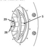
Pull the shoe 5 and its shim(s) 4, first in the radial direction to let pin come out of the rotor then out of the pump.
