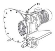
Fill the pump with corresponding volume of lubricant :
