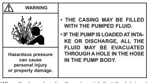
When the hose breaks, there is a risk that the lubricant may be contaminated by the pumped liquid.
