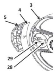
On rotor hub 19, loosen all screws without removing them. Put 5 screws in the extraction threading to loosen the hub.
