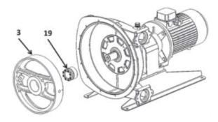
Position rotor 3 to have distance B between rotor outer edge and casing 1 back wall.
