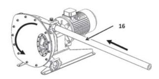
Rotate the pump intermittently until the hose 16 is completely inserted in the body and show equal lengths outside the body on both ports:
