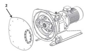
Screw and tighten screws 33 and their washers 34, starting by top ones to secure cover assembly.
