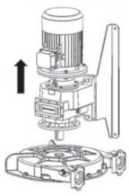
Remove shaft seal 26 from pump body. Put new shaft seal 26 in pump body.
