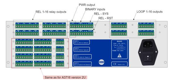
LOOP 1-16 outputs (A3716/3U only) contains 4-20 mA current outputs clamps.
