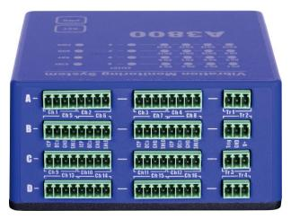
**Group A:** AC and DC channels 1-4, TACHO input 1. **Group B:** AC and DC channels 5-8, TACHO input 2. **Group C:** AC and DC channels 9-12, TACHO input 3. **Group D:** AC and DC channels 13-16, TACHO input 4.
