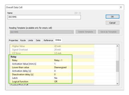
Relay – active relay where measurement is ongoing,
