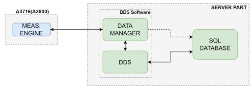
**MeasEngine** – Every online unit contains this software. It is performing measurements, collects data and provides them to Data Manager (part of DDS).
