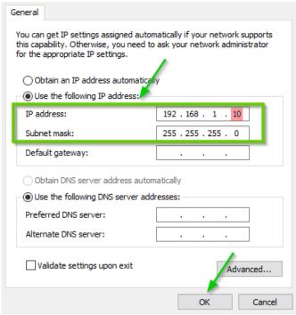
**3.Check connection between online unit and PC.** You can check this connection by using command line and "ping" test.
