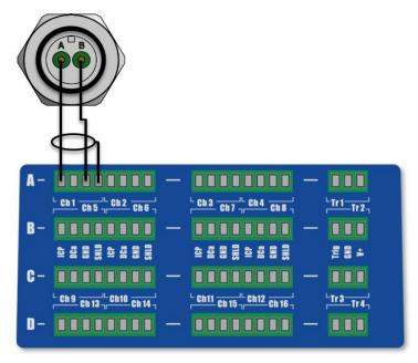
In case **ICP** is turned **OFF**, you will connect sensor as below (using input DCa, regardless of whether sensor is AC or DC – second connector for Ch1).:
