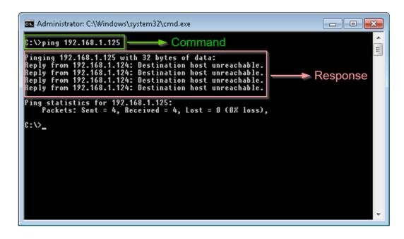
If you did not establish a connection with computer, make sure the computers (online unit and PC) are physically connected by a network cable. Check if the cable is not damaged. Furthermore, make sure that required IP addresses of computers are correct. If you still fail, contact the IT department.
