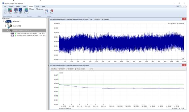
**Note:** There is "**Data transfer**" interval set by default to 180 seconds. This means it takes 180 seconds to send data from unit into database (you can see the first data after this interval).
