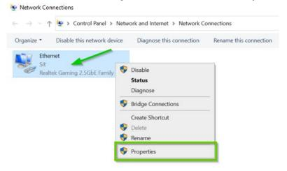
Choose option *TCP/IPv4* and click on *'Properties'*. Now you have two options how to set IP address for unit. First one is set it automatically with DHCP. See below.
