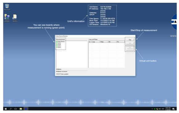
**Note**: You can see that button for Virtual unit is greyed in the picture. You can run virtual unit **only** when measurement in Online device monitor is **stopped**.
