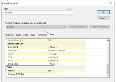
If measurements are set as Manual (value set to Yes), no measurement is performed automatically. Measurement starts only after pressing '**Start**' button (Online tab). Pressing of '**Stop**' button stops the collection of these data cells.
