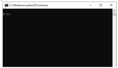
Enter command 'ping' with IP address of the online unit (for example ping 192.168.1.124). **If connection is successful**, this computer will respond with list of reply times (like in the picture below).
