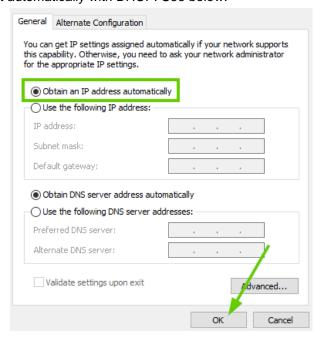
**Note**: If DHCP is used, IP address is assigned to online unit automatically from available range of IP addresses.
