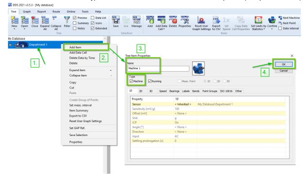
Measure points are created same way – click on Machine 1 with right mouse button, *difference*: type will be Meas. point. You need to choose measure point dimension (1D, 2D, 3D). It is important to choose Online unit (see picture below) and channel where sensor is connected. Channel 1 is first input of online unit.
