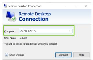
IP address from front panel of online unit could be (and most probably will be) different than the one obtained automatically. Remote desktop would not connect with IP address from production in this case. That is why you can login with units name.
