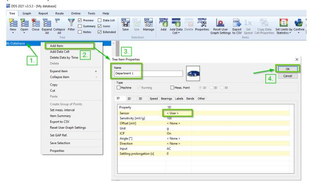
For sensor is important to set **sensitivity** [mostly used: 100 mV/g], **unit** [g] and **ICP**. ICP is set to value 'On' when sensor is connected and ICP powered – *in this case, keep in mind, that sensor needs to be correctly connected to online unit based on scheme in Sensor connection for unit A3800: first scheme.*
